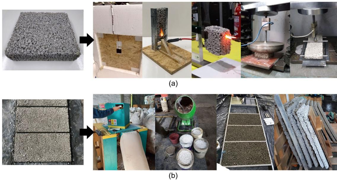
Figure 2. Developments and activities carried out in the laboratory and the cooperative: (a) Insulating material and technical tests based on international regulations; (b) Insulating plate product and production processes on a larger scale. Source: Preparation by the authors.
