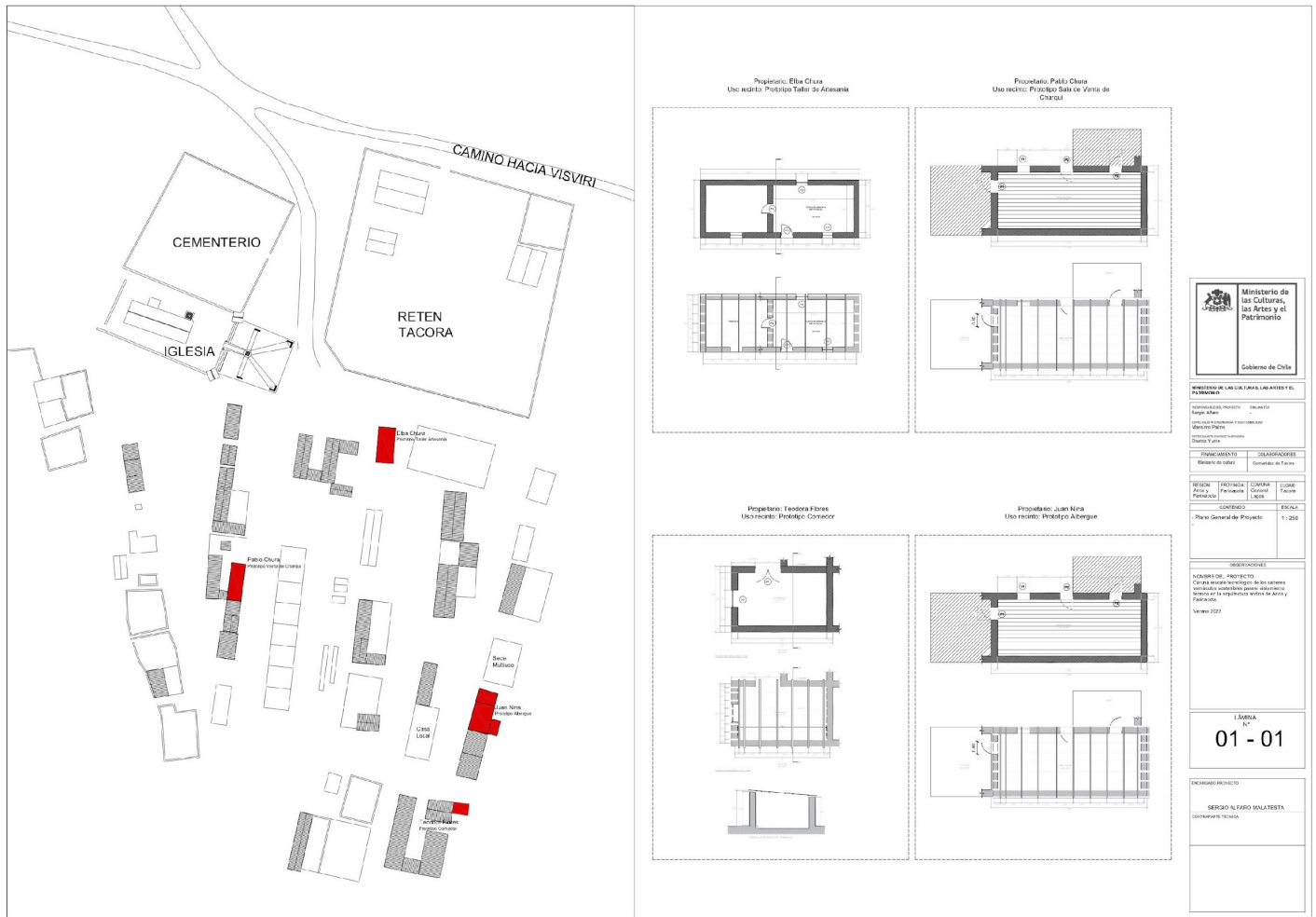
Figure 4. Plan of Tacora, August 2022, overview of the village, walls, and ceilings of houses considered for the indoor climate study. Source: Preparation by the authors
