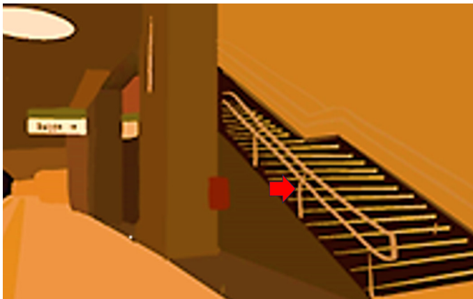
Figure 2a. Example of a staircase with double handrails on its edges. Source: Preparation by the authors
