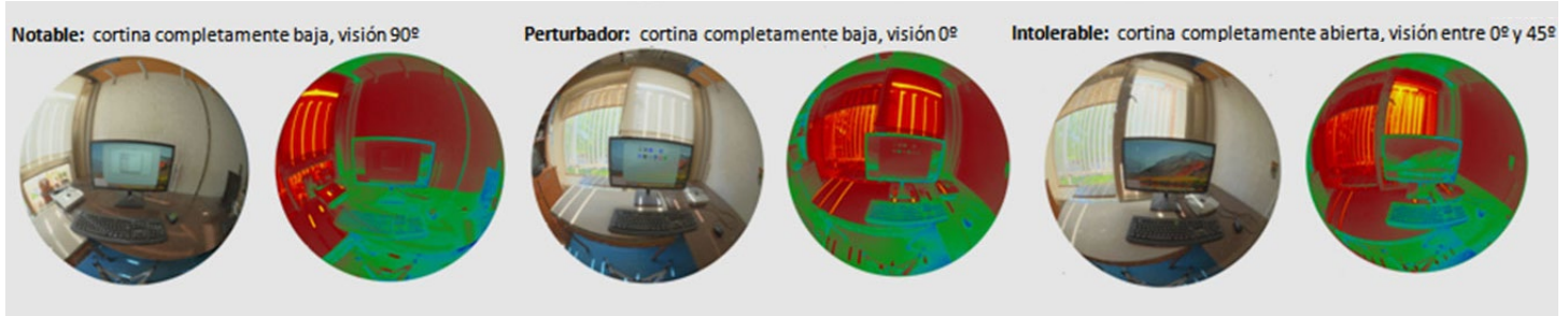
Figure 2. The six figures show an example of the three glare conditions generated by users when adjusting the roller blinds and monitor position on the desk. Only the right blind was adjusted. A photo was taken with a fisheye lens with a viewing angle of 180° to have a complete view of the surroundings. Source: Preparation by the authors.
