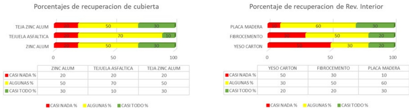
Figure 9. Roof and Interior Finish. Source: Preparation by the authors.
