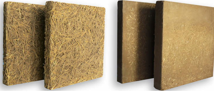
Figure 1: Test cell for the thermal test: a) Lightweight filler, b) Earth plaster. Source: Preparation by the authors.
