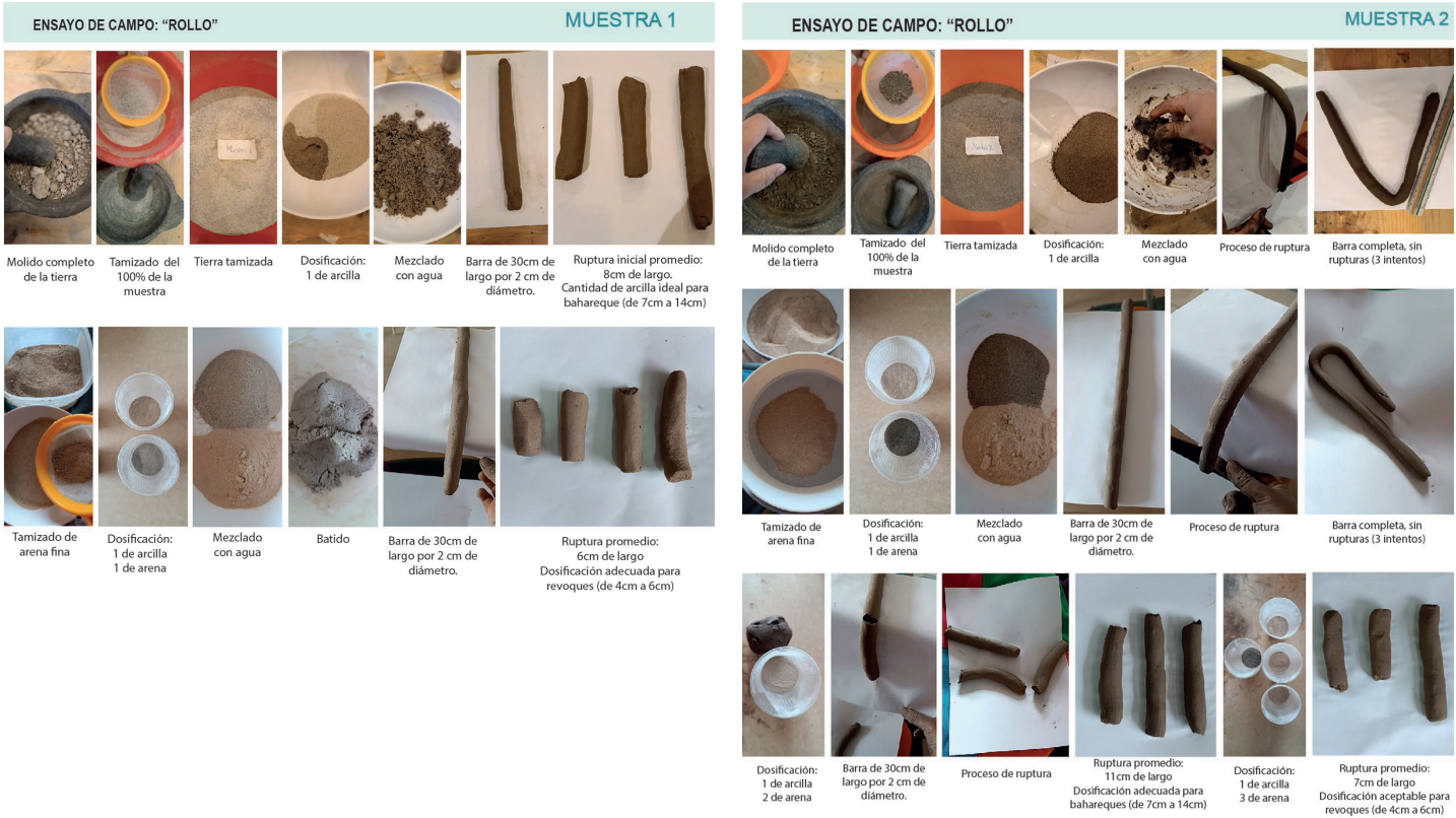
Figure 5. Roll-type field test (a) Sample 1; (b) Sample 2. Source: Preparation by the Authors based on Pahaut et al. (2020).
