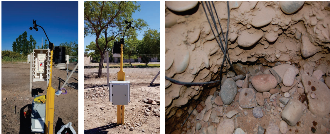
Figure 2. a) Weather Station b) Calibration c) Placement of thermocouples on the ground Source: Made by the author.
