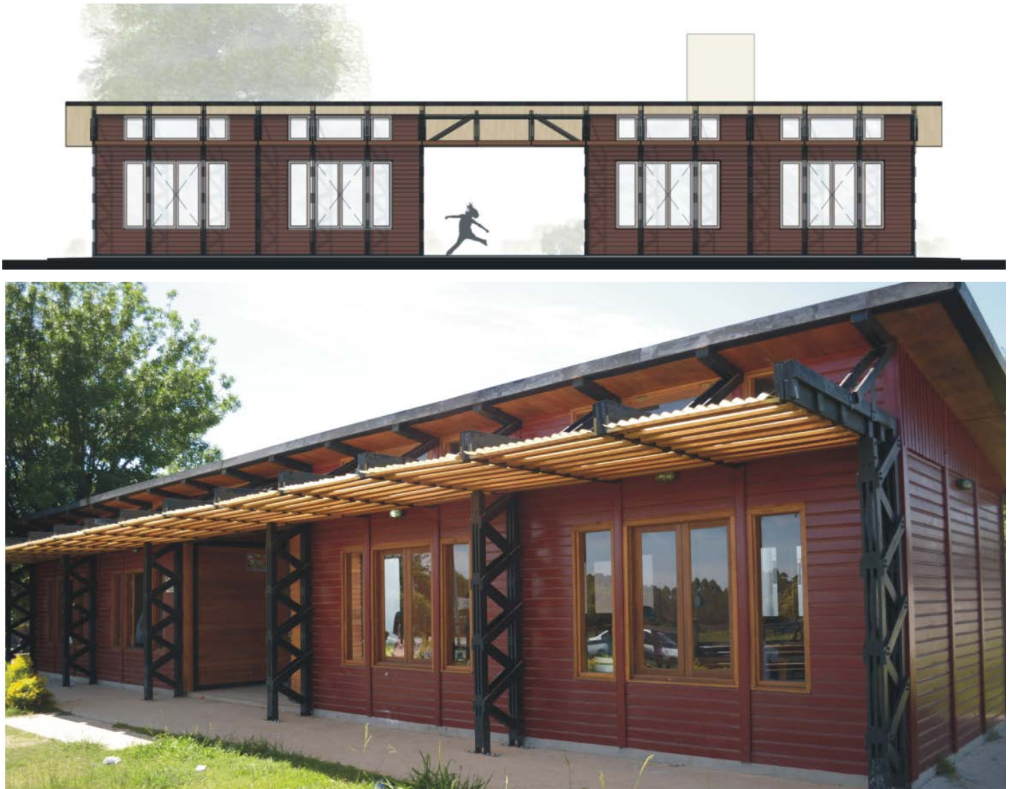
Figure 4. Design and technological development of a SUM with local wood. Source: Images extracted from PID 0079 (2016).
