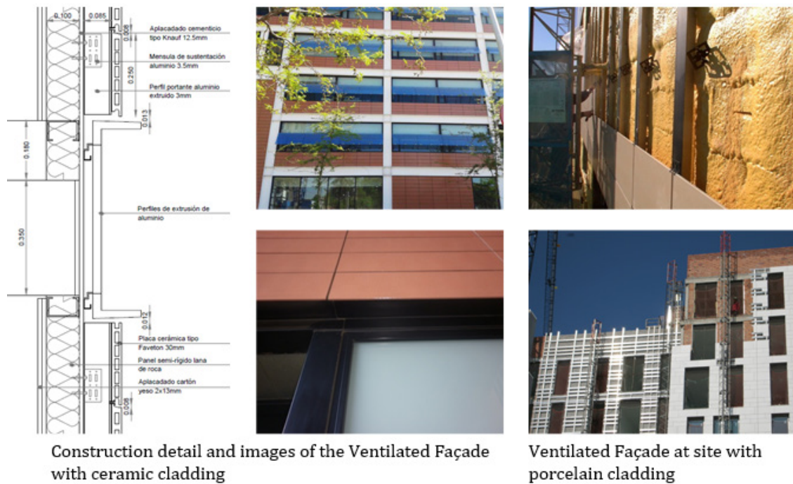
Figure 1. Different ventilated façade solutions in Barcelona, Spain. Source: Preparation by the Authors 1
