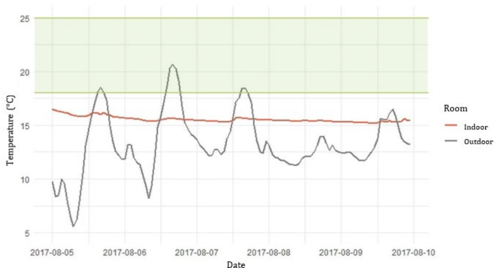
Figure 11. Outdoor and indoor temperatures in winter, without occupation. Source: Preparation by the authors in R.
