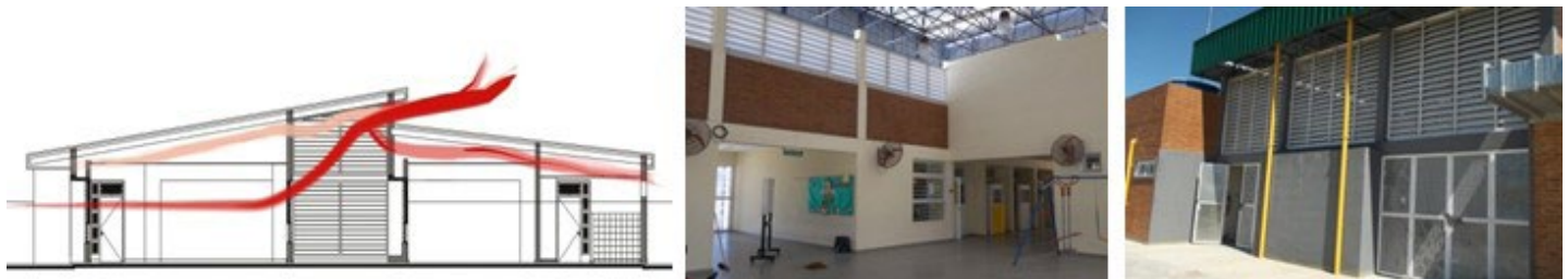
Figure 4. Natural ventilation layout. Interior and exterior photos of the SUM. JI 174. Source: Preparation by the authors.
