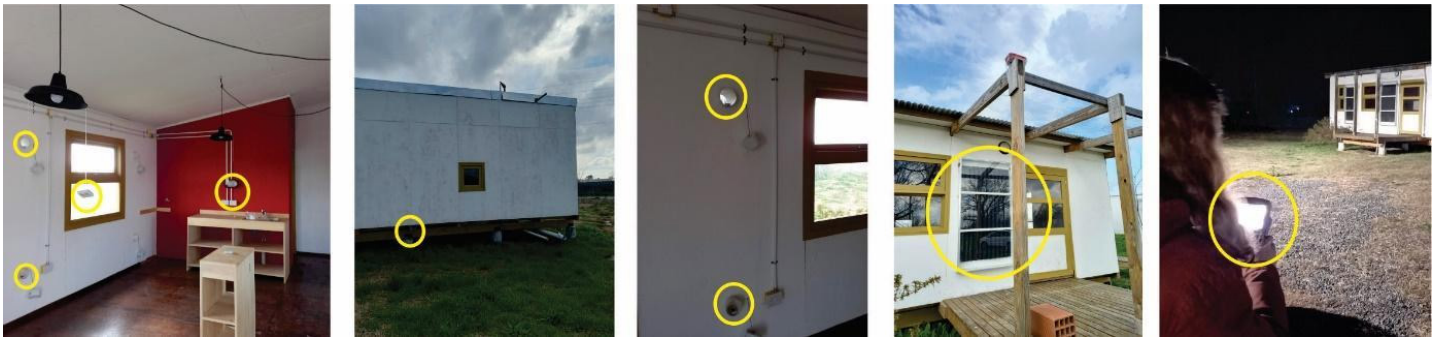
Figure 2. Placement of data loggers and thermographic imaging. Source: Preparation by the authors
