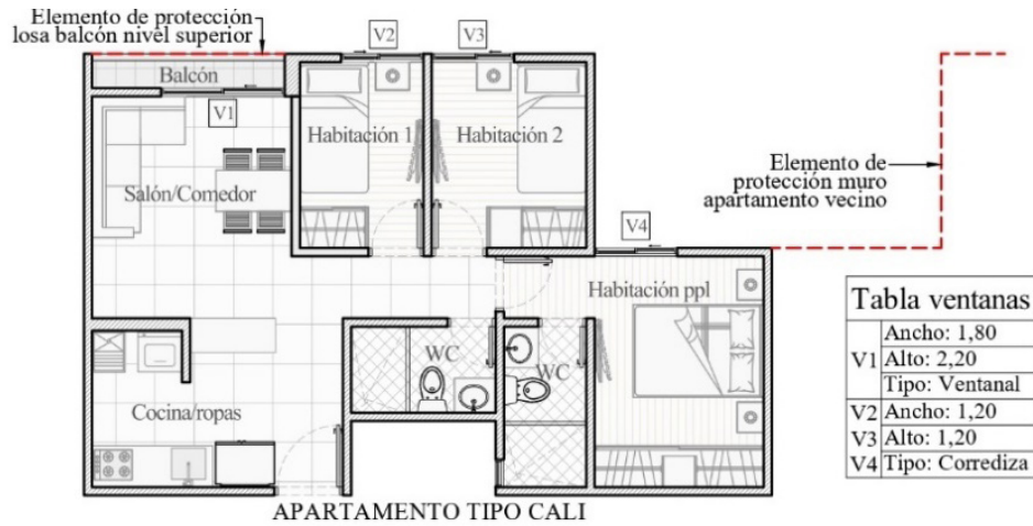
Figure 3. Architectural floorplans of standard housing for Cali, indicating the location of openings and obstructions. Source: Preparation by the authors.
