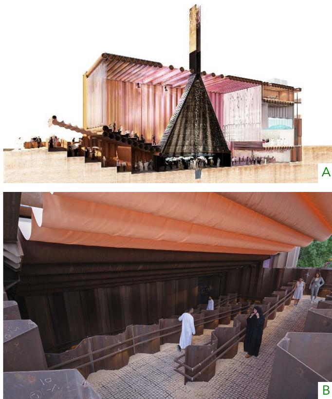
Figure 8. (A) Netherlands Pavilion 3D section showing materials, levels, and movement axis and (B) entrance gateway with a horizontal projection and leveling. Source: Aouf, 2021; The National UAE, 2020.
