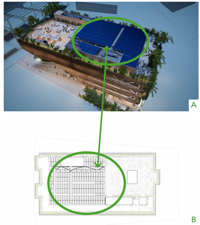
Figure 3. (A) Belgium pavilion’s perspective and (B) roof plan indicating solar canopy. Source: Assar, 2020; Dey, 2021.
