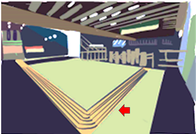
Figure 3a. Example of a complete connection of the tactile tread between the ticket office and the access to the turnstiles. Source: Preparation by the authors
