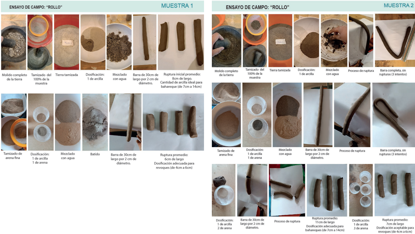
Figure 5. Roll-type field test (a) Sample 1; (b) Sample 2. Source: Preparation by the Authors based on Pahaut et al. (2020).
