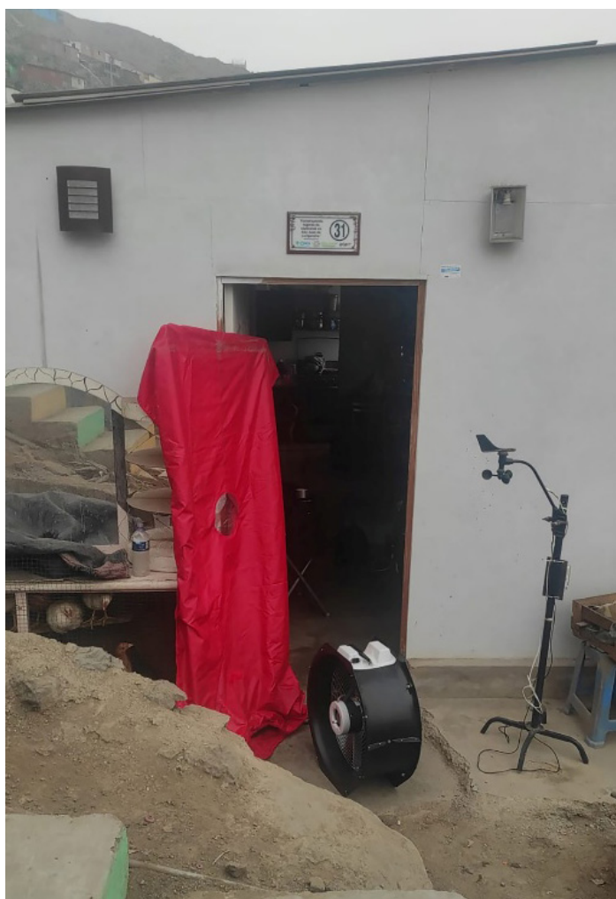
Figure 5. Left. Blower door installed in Dwelling V03. Source: Prepared by the Authors. Figure 6. Right. Sensors installed in Dwelling V02. Source: Prepared by the Authors.
