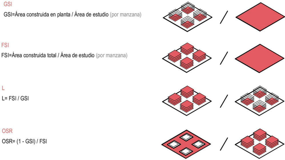
Figure 3. Outline for the calculation of the four indicators to classify morphologies. Source: Berghauer & Haupt, 2021.
