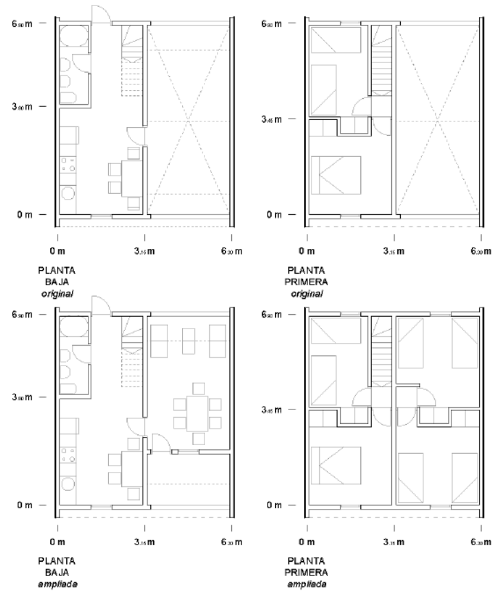
Figure 8. Housing unit designed by Elemental in Villa Verde and adopted by Group B. Source: Prepared by the authors based on Elemental's design.
